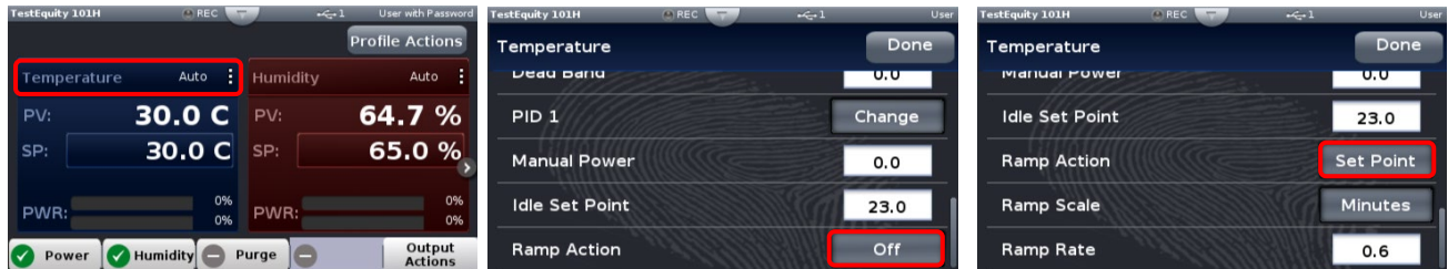
Ramp Action button is at the bottom of the loop screen. Off was changed to Set Point in this example.
